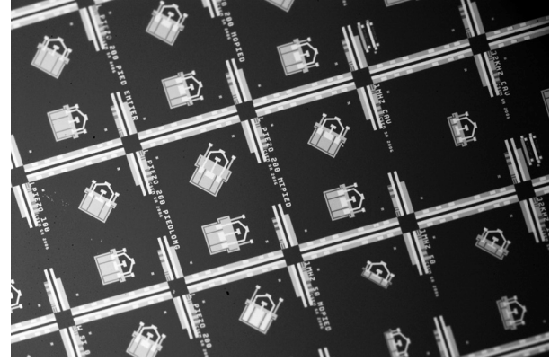
Figure 3. Top view of flexural resonators.
